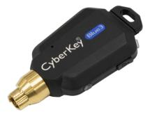
The CyberKey Blue 3 is an electronic key used to operate CyberLock cylinders and FlashLock access points. It has memory that contains encrypted access codes, a list of locks it may access, schedules of authorized dates and times it may access locks, and a begin-end date range during which the key will operate. The battery from a CyberKey energizes the electronics within a CyberLock cylinder.
