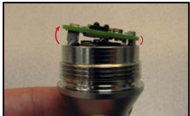
Figure 3: Skewed Circuit Board on Post
